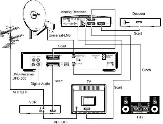
Connection of a DVB receiver to an analogue Sat receiver and the complete TV and hi-fi system. The digital sound output can be connected to a Dolby Digital System.
